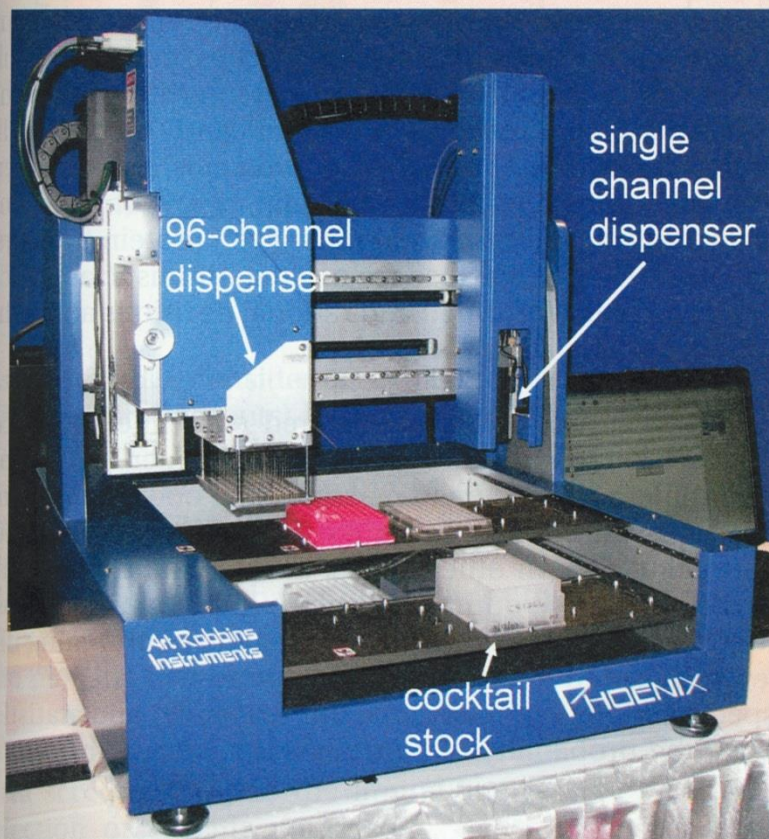
Figure 3-33 A robot for automated crystallization plate setup. The Phoenix robot (Art Robbins Instruments) can set up 96 crystallization trials in about one minute. On the left side, a 96-channel syringe dispenser re-arrays (100 \mu\text{l} each) 96 prefabricated or purchased crystallization cocktails simultaneously from a standard deep-well block into the reservoirs of an SBS-format, 96-well sitting-drop crystallization plate, and places between 1 \mu\text{l} and 100 \text{nl} into the drop shelves or wells. From the right side, a contact-less microvalve dispenser nozzle immediately adds the pre-aspirated protein (stock vials in the red block) rapidly and without contact onto each of the precipitant drops. To minimize evaporation, the plate is then immediately sealed with a sheet of pressure-sensitive adhesive. Taking all losses into account, about 12 to 15 \mu\text{l} of protein stock is required for 96 100 + 100 \text{nl} drops. The robot design has been based on a prototype developed in an academic laboratory setting. 84
