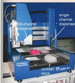
Figure 3-33 A robot for automated crystallization plate setup. The Phoenix robot (Art Robbins Instruments) can set up 96 crystallization trials in about one minute. On the left side, a 96-channel syringe dispenser re-arrays (100 \mu l each) 96 pre-fabricated or purchased crystallization cocktails simultaneously from a standard deep-well block into the reservoirs of an SBS-format, 96-well sitting-drop crystallization plate, and places between 1 \mu l and 100 nl into the drop shelves or wells. From the right side, a contactless microbubble dispenser nozzle immediately adds the pre-aspirated protein (stock vials in the red block) rapidly and without contact onto each of the precipitant drops. To minimize evaporation, the plate is then immediately sealed with a sheet of pressure-sensitive adhesive. Taking all losses into account, about 12 to 15 \mu l of protein stock is required for 96 (100 \times 100 nl) drops. The robot design has been based on a prototype developed in an academic laboratory setting. 34
